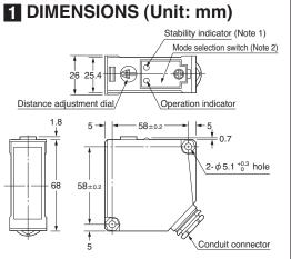
Notes: 1) It is the beam-receiving indicator for the **MR3-T**. 2) **MR3-T** incorporates a mode selection switch and timer adjustment dial.
